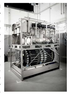
technology matures and the costs of its production technologies decrease. This talk will present some of the industrial progress related to the large-scale deployment of modular pressurized alkaline electrolysers.
