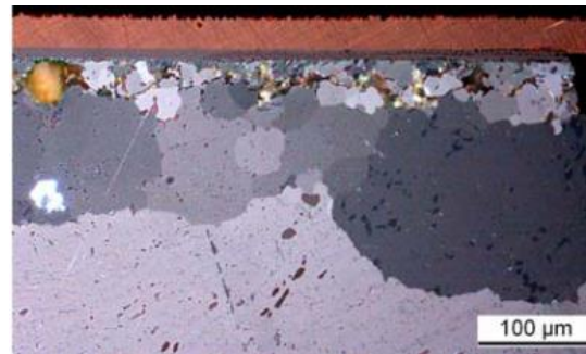
Grain refinement solder joint (pb-free) –thermal cycling
