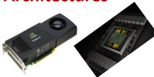
Accelerators high compute density, high performance/watt >9.7 TFlop DP on a chip
