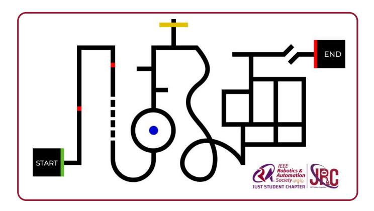
The beginning of the route is marked by a black **25 cm\*25 cm** square, and a **3 cm** green line wide in the front. Before starting the round, the robot should be placed in the black square and not touching the green line.
