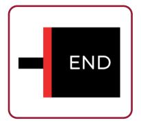
The route does not run closer than **15 cm** to the edge of the track, measuring from the edge of the line marking the route.
