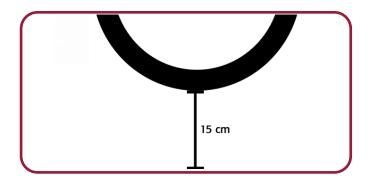
Two adjacent lines of the route do not run closer than **15 cm** from each other, measuring from the center of the line marking the route.
