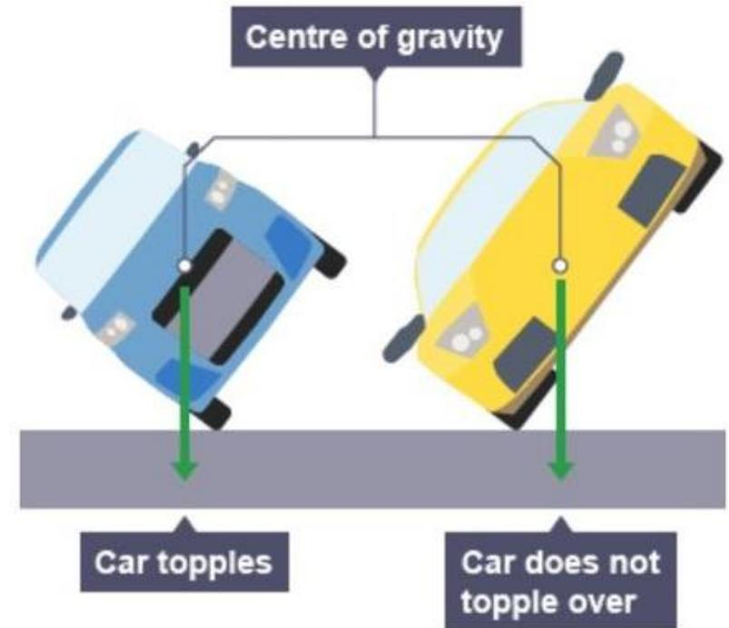
The wider car will not topple over because it has a lower centre of gravity, but the narrow car will
