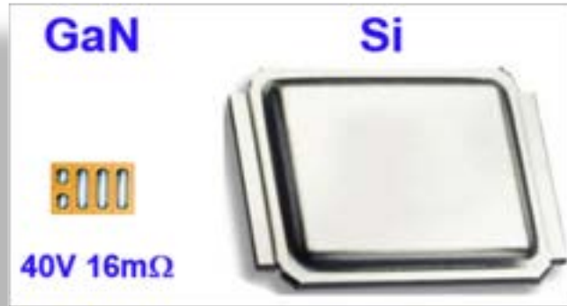
Size comparison of Si power MOSFET with GaN HEMT from EPC for same performance
