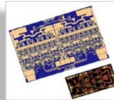
Size comparison of RF HEMTs based on GaAs and GaN technologies from Qorvo
