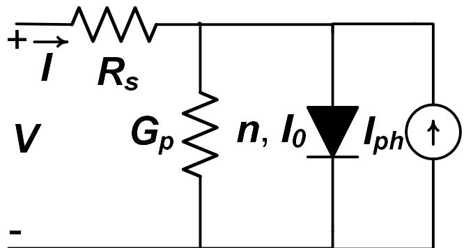
$$I = \frac{n v_{th}}{R_S} W \left\{ \frac{I_0 R_S}{n v_{th} (1 + R_S G_P)} \exp \left[ \frac{V + R_S (I_0 + I_{ph})}{n v_{th} (1 + R_S G_P)} \right] \right\} + \frac{V G_P - (I_0 + I_{ph})}{1 + R_S G_P}$$
