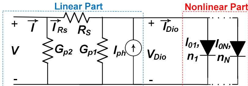
$$I = \left\{ \sum_{k=1}^N I_{0k} \left[ \exp \left( \frac{V - R_s (I - G_{p2} V)}{n v_{th}} \right) - 1 \right] \right\}$$
