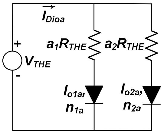
$$I_{Dioa} = \frac{n_{1a}v_{th}}{a_1R_{THE}}W_0 \left[ \frac{a_1R_{THE}I_{01a}}{n_{1a}V_{th}} \exp\left(\frac{V_{THE} + a_1R_{THE}I_{01a}}{n_{1a}v_{th}}\right) \right] - I_{01a}$$
