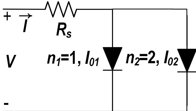
$$I = I_{01} \left[ \exp\left(\frac{V - I R_s}{v_{th}}\right) - 1 \right] + I_{02} \left[ \exp\left(\frac{V - I R_s}{2 v_{th}}\right) - 1 \right]$$
