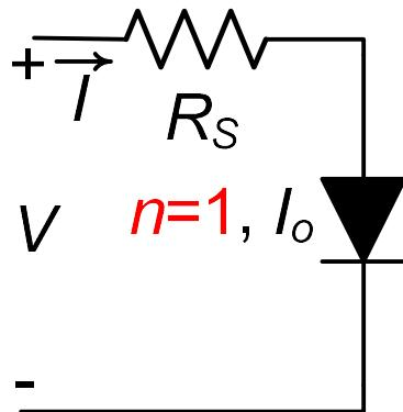
This method contains clever mathematical ideas and it was developed for Schottky diodes with  $n=1$ . The following notation is adapted to p-n junctions.
