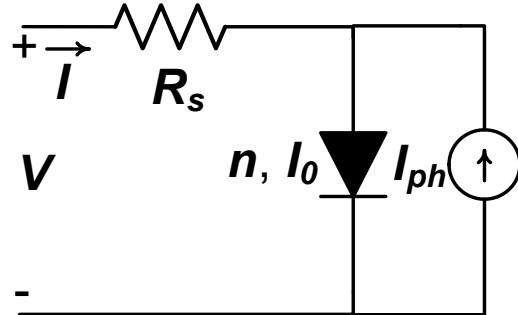
$$V = +I R_S + nV_T \ln\left(\frac{I + I_{ph}}{I_0} + 1\right)$$
