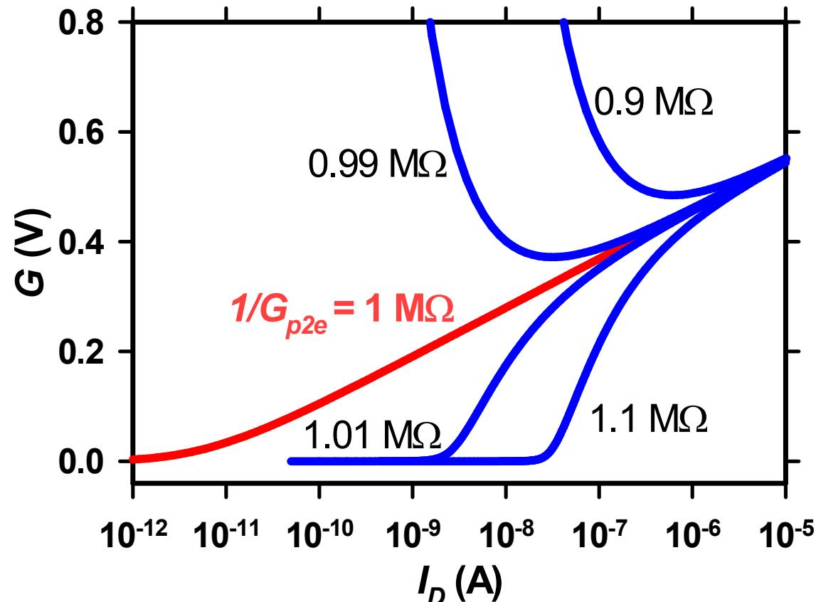
$G_{p2}$  is the value of  $G_{p2e}$  for which the graph of  $G$  vs  $I_D$ , is a **straight line**.
