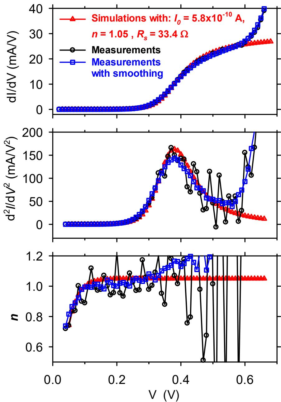
The differentiation method is successful with simulated data and it fails with measurements.
