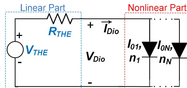
Applying Thevenin's theorem to the linear components:
