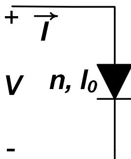
$$I = I_0 \left[ \exp\left(\frac{V}{n v_{th}}\right) - 1 \right]$$
