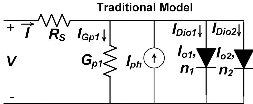
$$I = I_{01} \left[ \exp\left(\frac{V - R_S I}{n_1 v_{th}}\right) - 1 \right] + I_{02} \left[ \exp\left(\frac{V - R_S I}{n_2 v_{th}}\right) - 1 \right] - I_{ph} + G_{P1}(V - R_S I)$$
