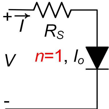
$$I = I_0 \left[ \exp\left(\frac{V - I R_s}{v_{th}}\right) - 1 \right] \quad (1)$$
