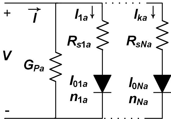
By solving each branch separately and adding the solutions, the alternative model presents analytical solution for the current:
