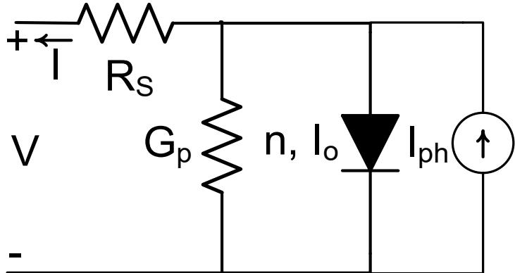
This case does not have analytical solution for the maximum power point.
