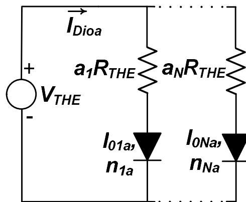
By solving each branch separately and adding the solutions, the alternative model presents analytical solution for the current:
