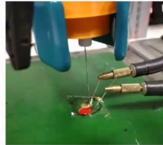
Microscale electrode modified with different electrocatalytic materials (e.g. Unimol, CV, and Cu)
